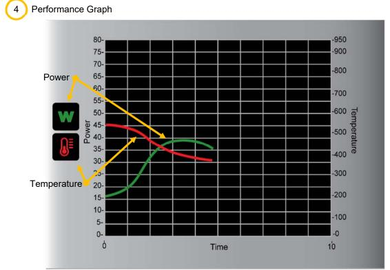
The Performance Graph displays the power and temperature from the initiation of a solder event for each solder joint. Selecting the Power or Temperature icons will enable or disable the display of the parameter.
