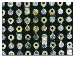
Open via and solder resist damage.
