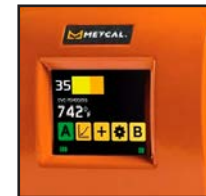
Tip temperature displayed on large color screen.
