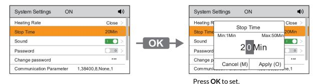
The Stop Heating Time is 20 minutes. Press on the Main Interface to start heating and display a countdown of 20 minutes and 0 seconds. After the end of the timer, the device will automatically turn off the heater. Press again to restart the heating and countdown.
