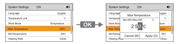
Note: Temperature upper and lower limits can restrict the maximum and minimum ranges of the unit's temperature settings. The factory default temperature upper limit is  $250\,^{\circ}\text{C}/482\,^{\circ}\text{F}$ . The default temperature lower limit is  $50\,^{\circ}\text{C}/122\,^{\circ}\text{F}$ . The adjustable range is  $80\,^{\circ}\text{C}$  to  $50\,^{\circ}\text{C}$  ~ $250\,^{\circ}\text{C}$  /122 °F ~ $482\,^{\circ}\text{F}$ .
