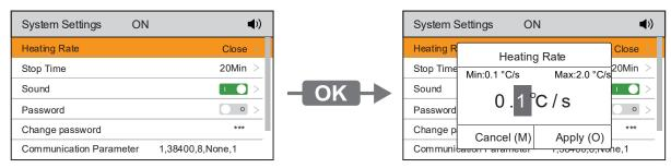
The current heating rate is set to 0.1 °C/s. When the device is heated, it will heat up by 0.1 °C per second
