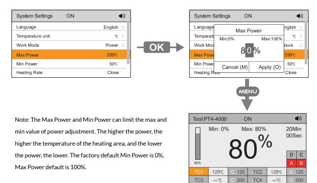
The current min power can be set to 0% and the max power can be set to 80%.
