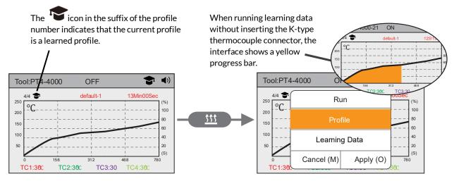
Press to select **Run Profile** to run the current profile. **Run Learning Data** can also run without inserting the K-type thermocouple connector.
