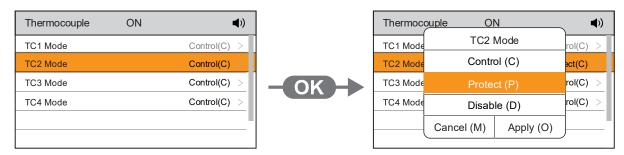
**Example:** TC2 is in (P) Protection Mode. When the specified temperature is reached, heating stops.
