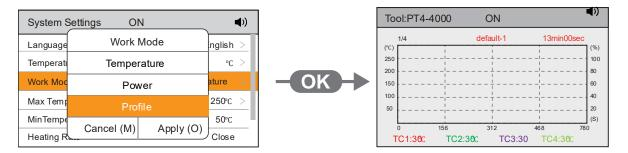
Press ▼ or ▼ to switch the curve in the Main Screen. The curve cannot be switched while it is running.
