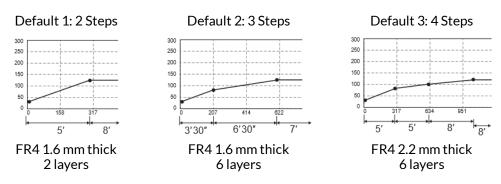
Profiles set using the lowest height position of the BH-4000 Board Holder (18 mm between PCB & heating area.
