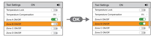
Example: Heating Zones A and B are in the enabled state.
